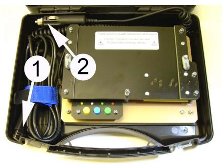
SCU Unlock Tool After Upgrade (1) USB Connector: For PC control, not needed when used in 'stand-alone' mode , when the cigar lighter plug (2) can be used instead
